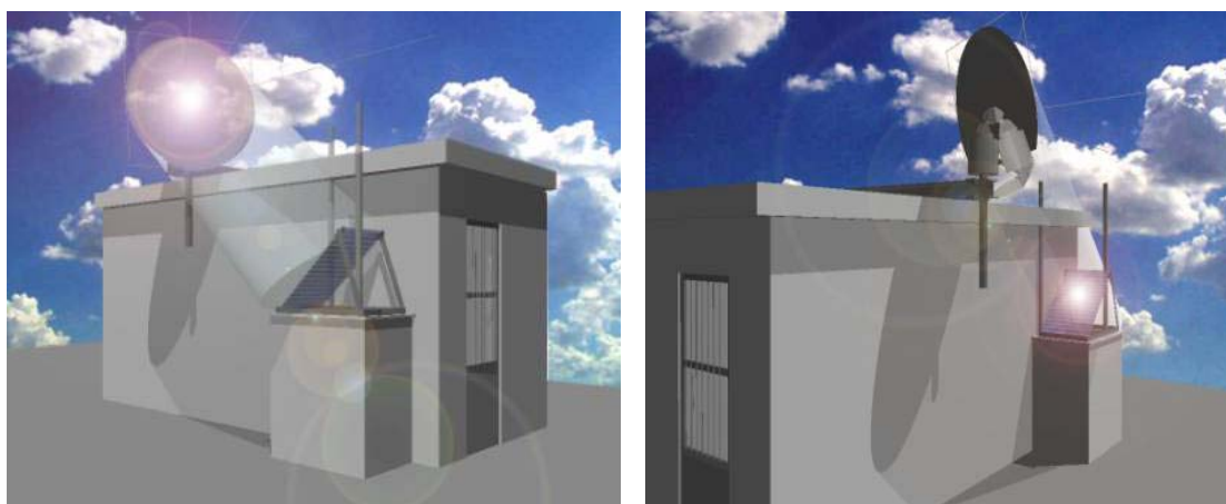
Figure 4 Light Shaft with White-Light-Holograms and heliostat in Athens
